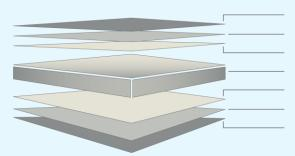
Finish Coat (Finish Coat + Primer = nominal 25um) {Refer Notes 4 & 5} Universal Corrosion Inhibitive Primer
